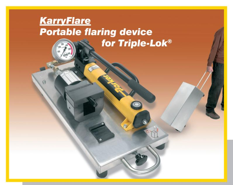
The KarryFlare is a portable device for easy and workmanlike 37° tube flaring. It allows the flaring of even large dimension steel and stainless steel hydraulic tube at assembly sites where Parflange<sup>®</sup> technology is not available.
